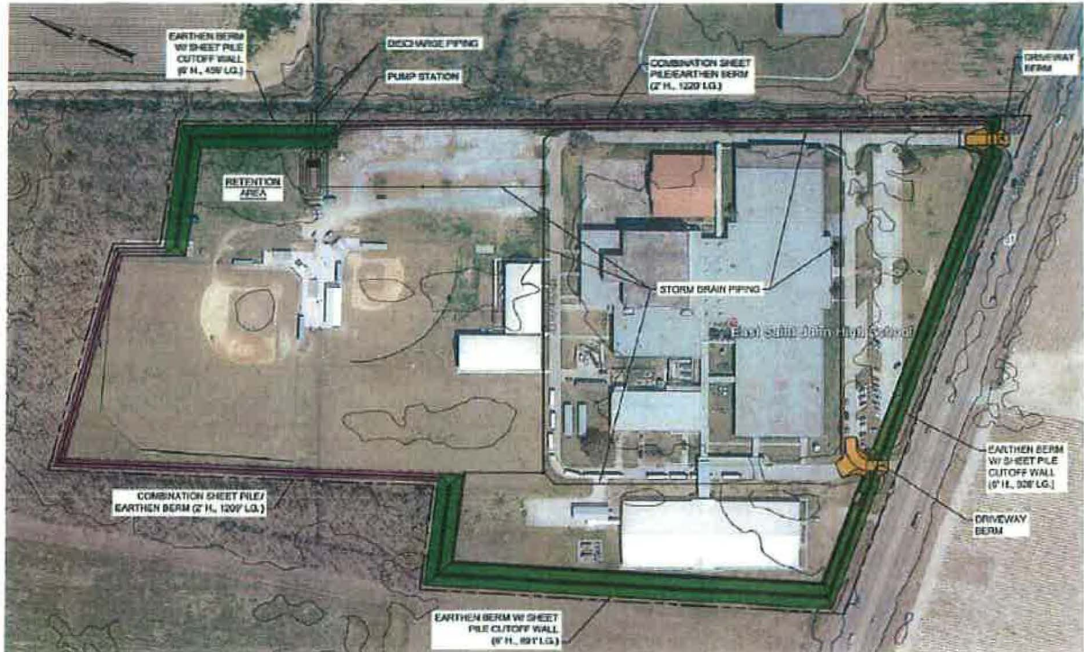
Schematic design for floodwall, provided by the applicant
