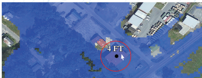
The example illustrates how to determine a BFE in Zone A using the WSEL grid. This procedure can be used to determine if it might be appropriate to apply for a Letter of Map Amendment (LOMA).
