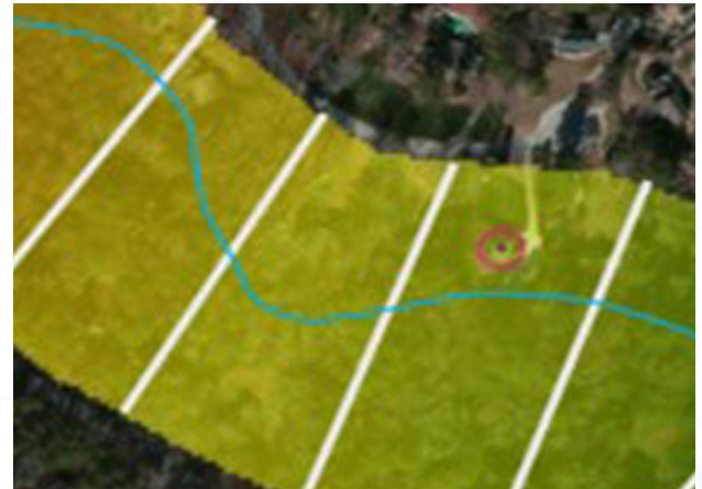
The estimated BFE can be cross checked against the water surface elevation data found in flood model cross sections, if available.
