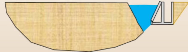
4 - Embankment continues to scour and cannot be stopped
