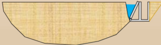
3 - Embankment starts to scour
