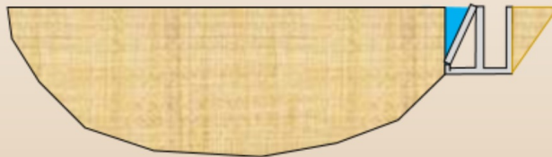
2 - Earthquake damages spillway wall producing upstream to downstream seepage path
