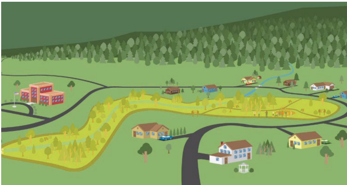
Figure 10. Hazardous fuel maintenance can be incorporated into community landscaping and design to provide protection against the spread of wildfire in open spaces, parks, recreational areas, and man-made drainages (U.S. Fire Administration, n.d.).
