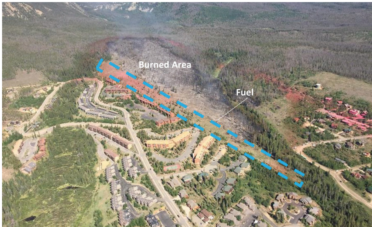
Figure 13. Fuel breaks (the blue line between the homes and forested area) played an important role protecting homes during the 2018 Buffalo Fire in Summit County (U.S. Forest Service).
