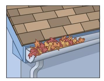
Figure 1. Debris in gutters can ignite and lead to ignition of roof or fascia board.
