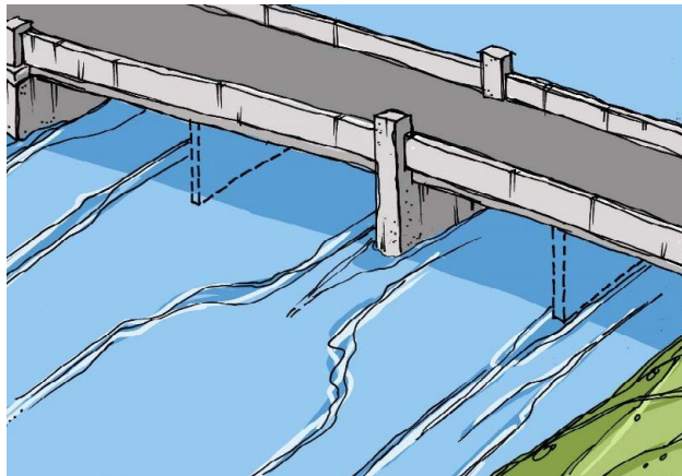
Figure 1.4.2. Reducing the number of spans can increase the flow amount under the bridge. In this figure, the dashed piers would be removed to accomplish this.
