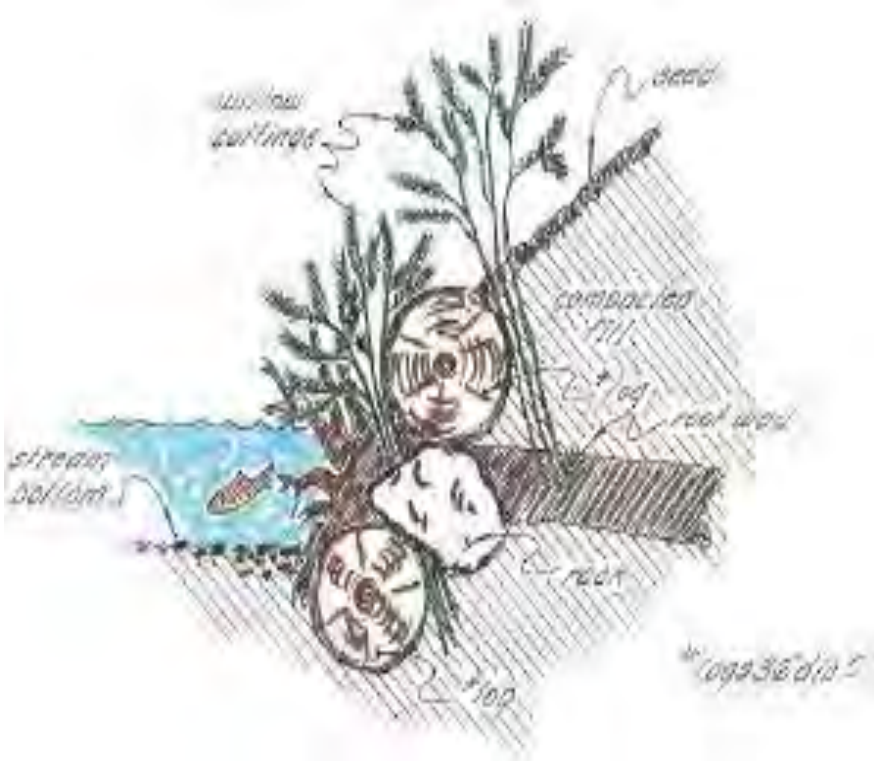
Figure 4-5: Woody Debris Bank Stabilization Cross-Section
