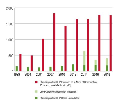
Figure 11. Number of State-Regulated High Hazard Potential Dams That Have Been Remediated or Other Risk Reduction Measures Utilized During the Reporting Period Because of Hydraulic/Structural Deficiencies
