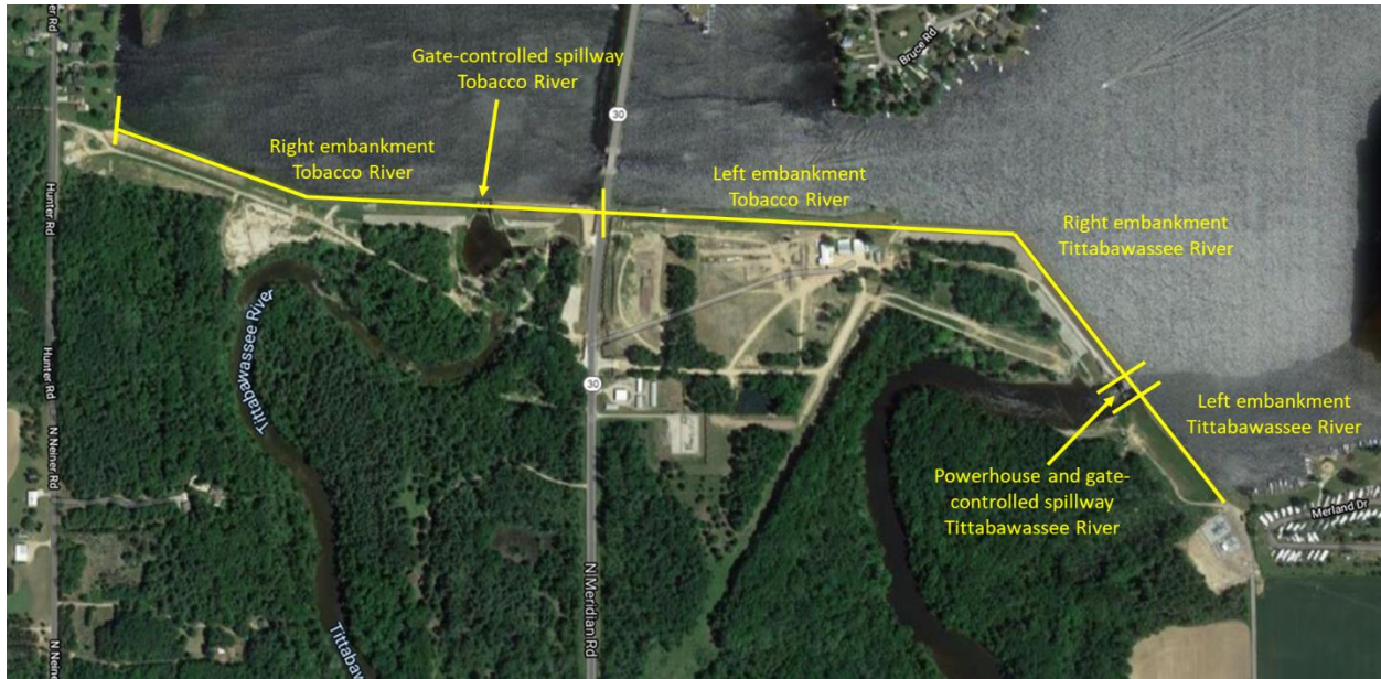
Figure 2: Main sections of Edenville Dam (left to right, looking downstream)
