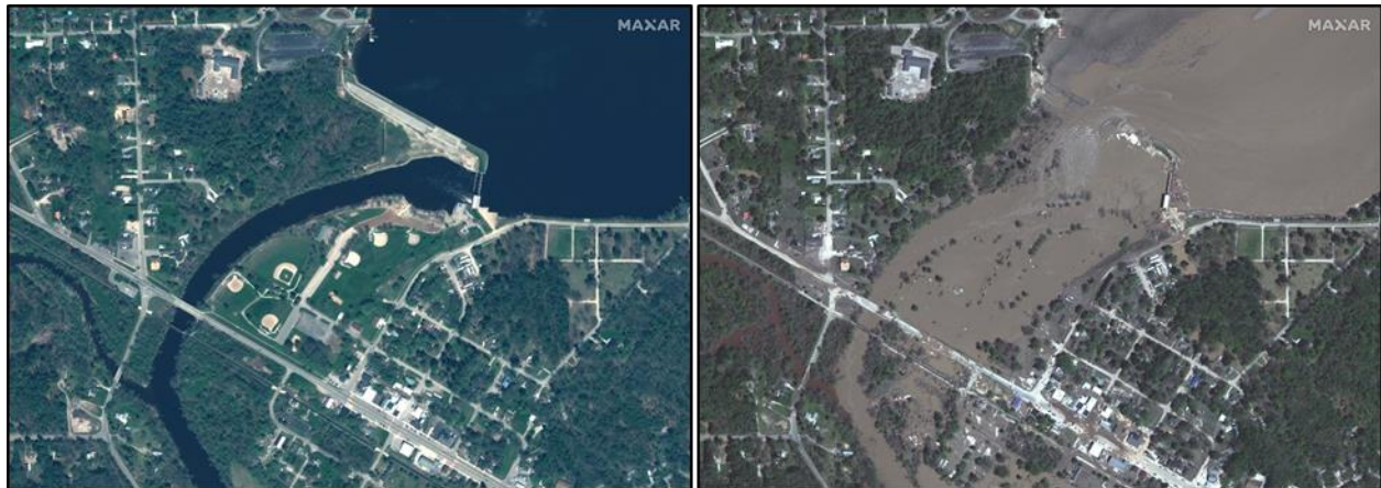
Figure 13: Sanford Dam: Aerial imagery before and after the dam failure (left, May 2019, and right, May 21, 2020) (Wilkinson/Maxar 2020)
