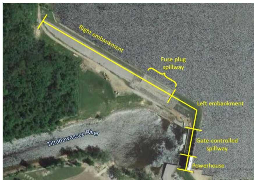
Figure 3: Main sections of Sanford Dam (left to right, looking downstream)
