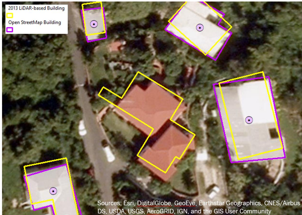
Figure 3-15: Example of a Lidar-Based Footprint Not Identified by OSM
