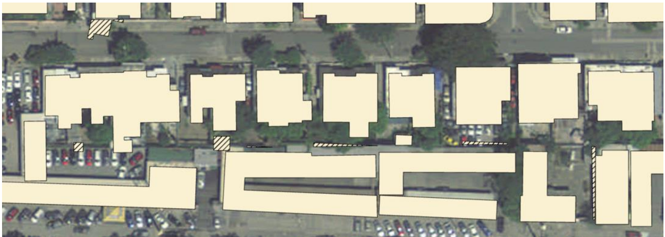
Figure 3-12: Example of Non-Existing Building Polygons Identified
