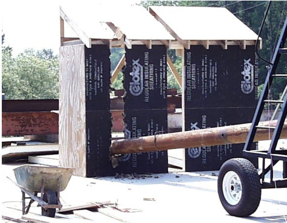
Figure 5-71 Large Pipe Impacting Roof and Wall Without Plywood Sheathing, 7,600 foot-pound at Impact, Breaking Roof, Top Plates and Entire Wall with Apparent Residual Energy Hitting Ground
