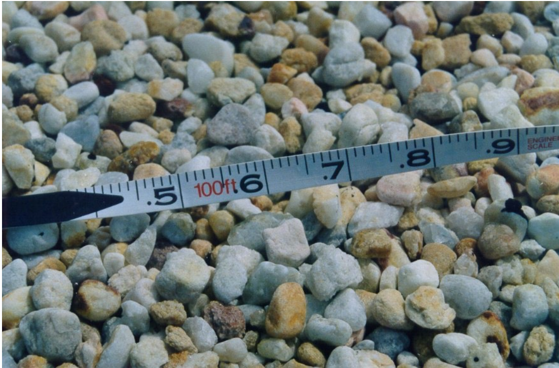
Figure 5-56 Roof Gravel on the Upstream Building
