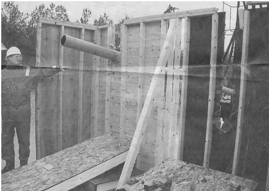
Figure 5-70 Small Pipe Impacting Wall with Plywood Sheathing, 3,600 foot-pounds at Impact, Breaking Top Plates and 1/4 Cutting Into Wall
