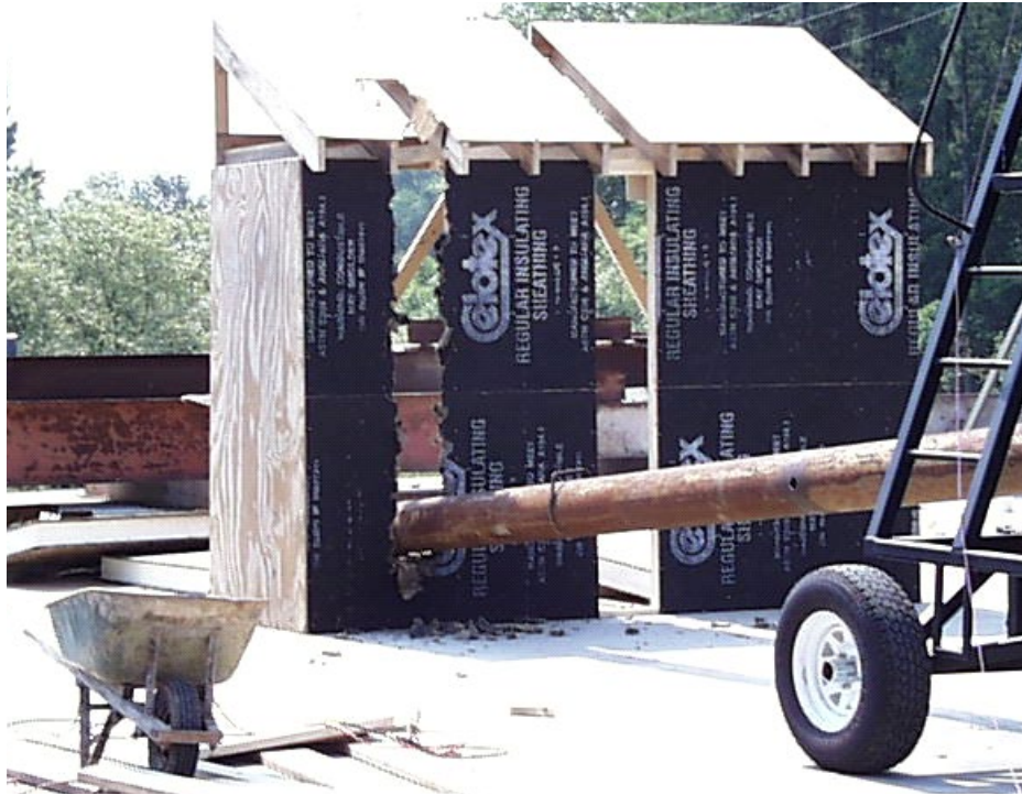
Figure 5-71 Large Pipe Impacting Roof and Wall Without Plywood Sheathing, 7,600 foot-pounds at Impact, Breaking Roof, Top Plates and Entire Wall with Apparent Residual Energy Hitting Ground
