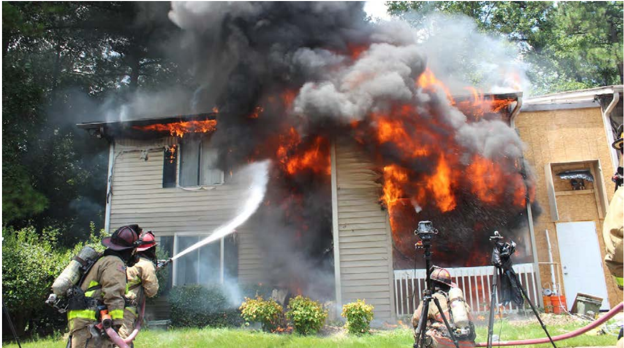
Figure 2: Fire conditions at the start of exterior fire control after horizontal ventilation at one of eleven Phase II apartment fire experiments.
