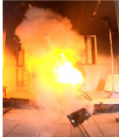
Figure 9: Casing of a 94 Ah cell flies apart as battery cell material inside burns in a fireball
