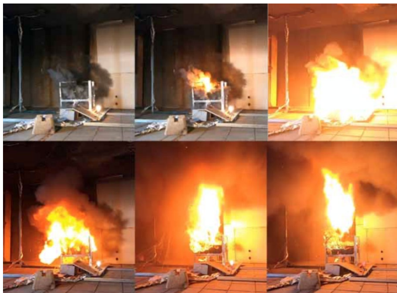
Figure 11: Sequential images of the failure of the first 94 Ah module cell in a rack mounted case containing 14 modules. Continued fire propagation and growth is displayed in the video 5 .
