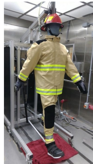
Figure 2. Fully dressed physiological manikin wearing turnout suit
