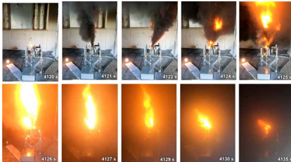
Figure 10: Images of the 94 Ah single cell during the intense venting and burning period lasting about 10 seconds.
