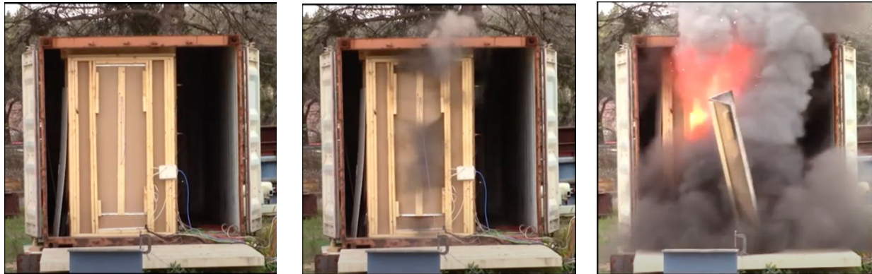
Figure 12: Sequential of images from the test video 6 showing the short time from the venting of gases from the failed 94 Ah module to explosion blowing the door off the closet. Image (Time 0 seconds): exterior view of the enclosure at the time the battery module begins to vent gases. Image (Time 3 seconds): first exterior visual evidence of venting. Image (Time 5 seconds): closet door blown away from the structure when accumulated combustible gases ignite.
