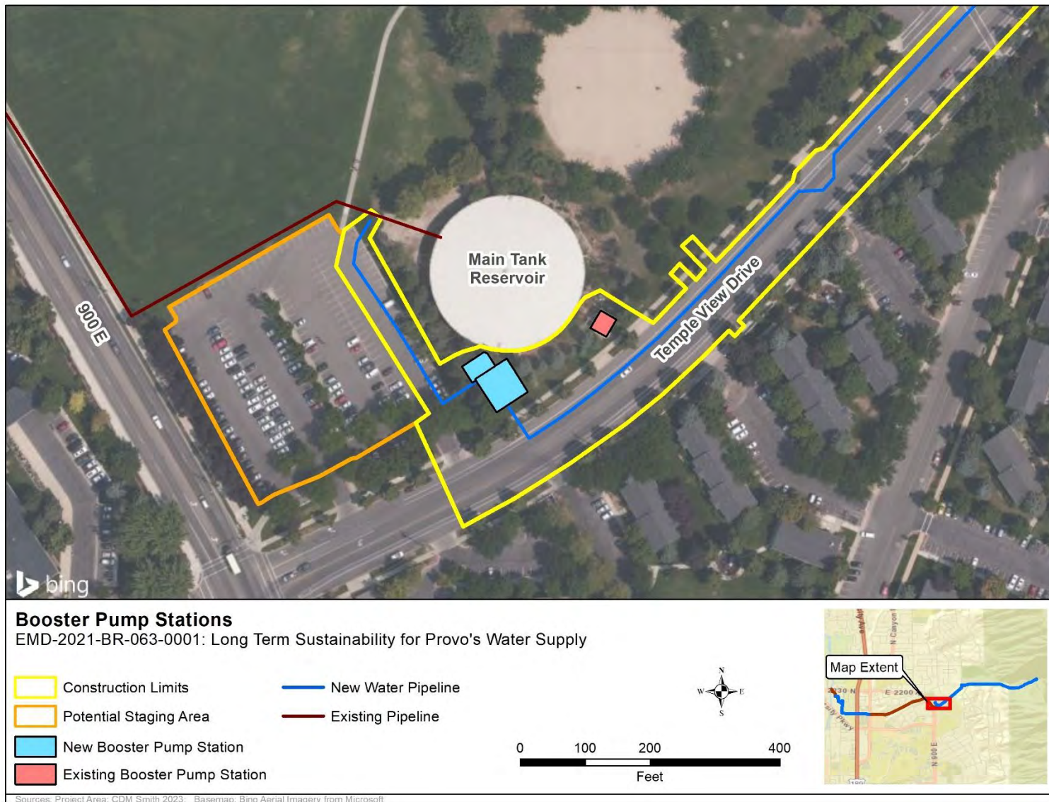
Figure 3-2. Proposed Booster Pump Station
