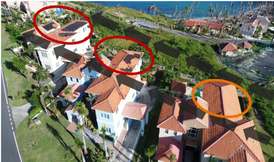
Figure 12. Visible severe (red) and moderate (orange) topographic wind speed impacts in Puerto Rico. Photo by Stuart Adams.
