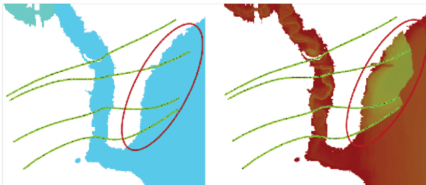
Figure 9: WSEL Grid Errors Resulting from Untrimmed Cross-Sections
