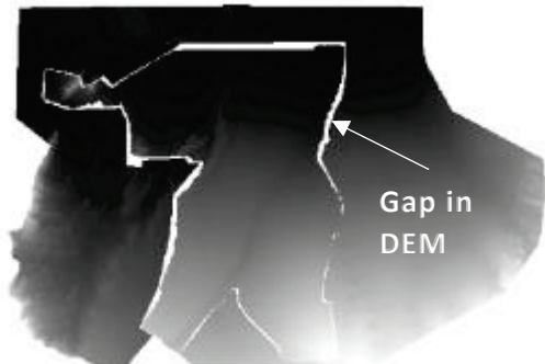
The gap represented above may exist between differing surveys and may therefore also cause gaps with WSEL, Depth and Analysis Rasters.
