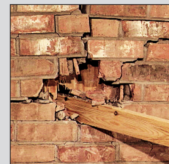
Design missile is 15 lb 2x4 traveling at 100 mph. Two laser timing gates provide verification of the recorded missile speed.
