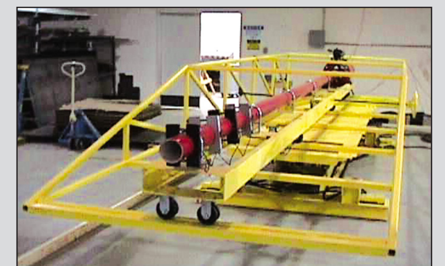
The new debris launch facility allows for a greater range of motion of the barrel and more accurate missile impact.
