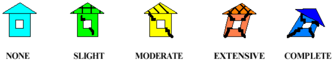
Figure 7-2 The Five Damage States
