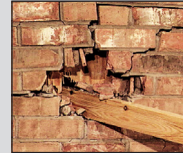
Design missile is 15 lb 2x4 traveling at 100 mph. Two laser timing gates provide verification of the recorded missile speed.
