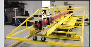
The new debris launch facility allows for a greater range of motion of the barrel and more accurate missile impact.
