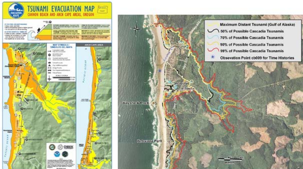
Figure 4.7: A tsunami evacuation map for the town of Cannon Beach, Oregon. (Left: two scenarios, distant and local events. Right: inundation map with inundation zones for distant and local tsunamis.
