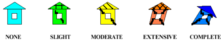
Figure 7-2: The Five Damage States
