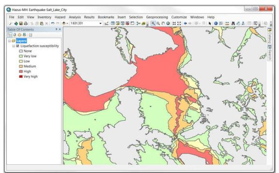
Figure 2.6: Example Liquefaction Susceptibility Dataset for the Wasatch Front, Utah
