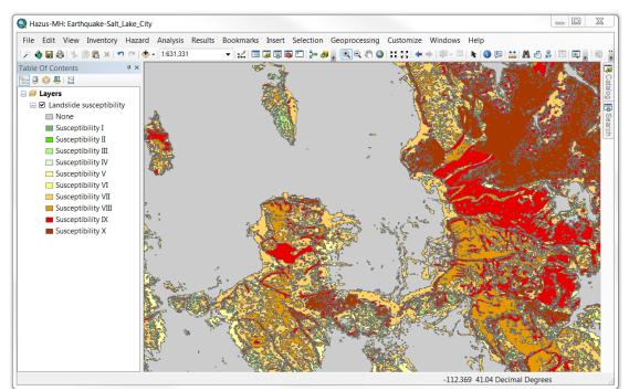
Figure 2.4: Example Landslide Susceptibility Dataset for the Wasatch Front, Utah
