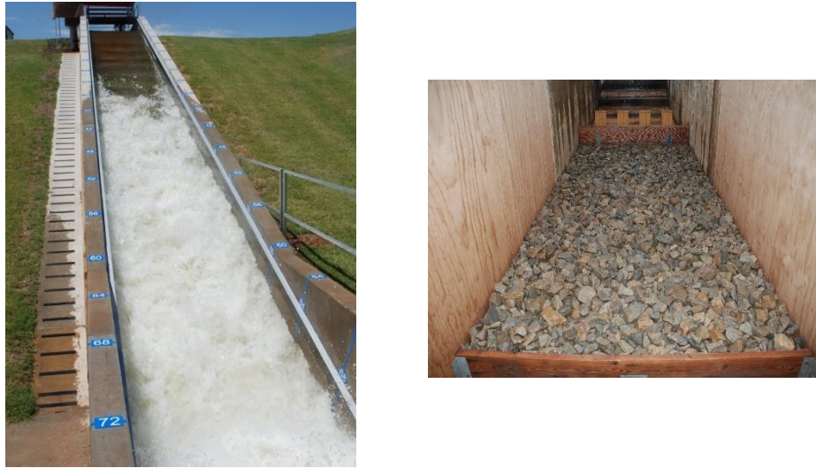
Figure 17 – Large scale flume of a stepped chute study on the effects of stilling basin design and downstream rock apron.
