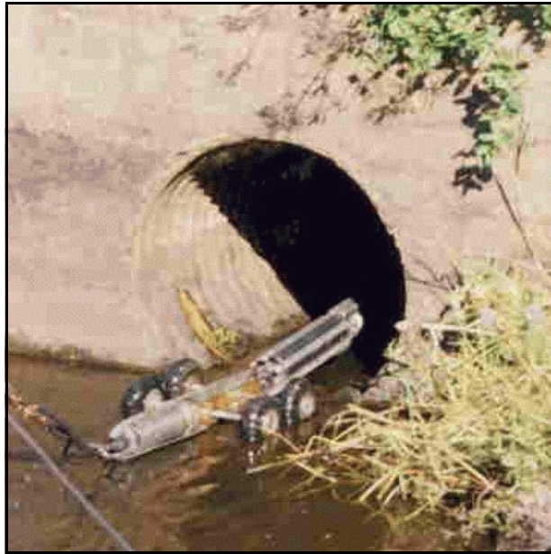
Figure 128. —A CCTV inspection camera-crawler entering the downstream discharge portal of an outlet works conduit.
