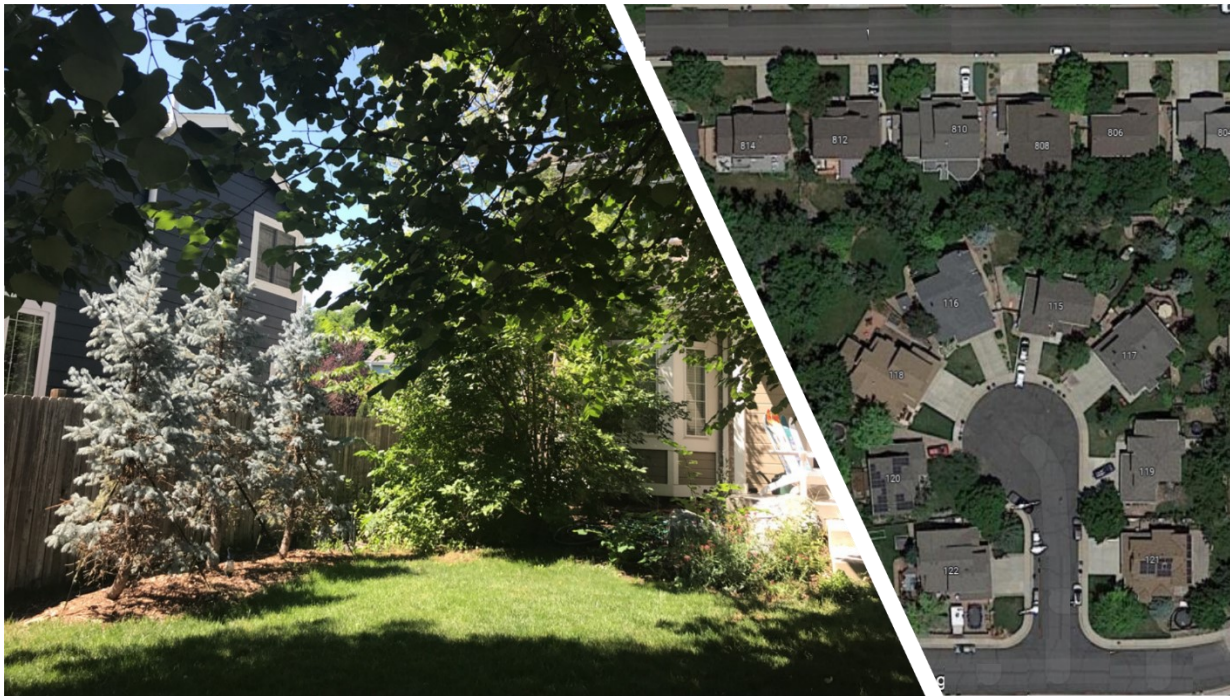
Figure 21. Example of single-family residences in Louisville, Colorado with 5–8 feet to the respective property lines (right) and significant overgrown vegetation typical within Zone 0 and 1 of both homes’ defensible space zones (left). Both homes are vulnerable to spot fires from embers or structure-to-structure fire spread due to poor vegetation management in the mutually shared defensible space.
