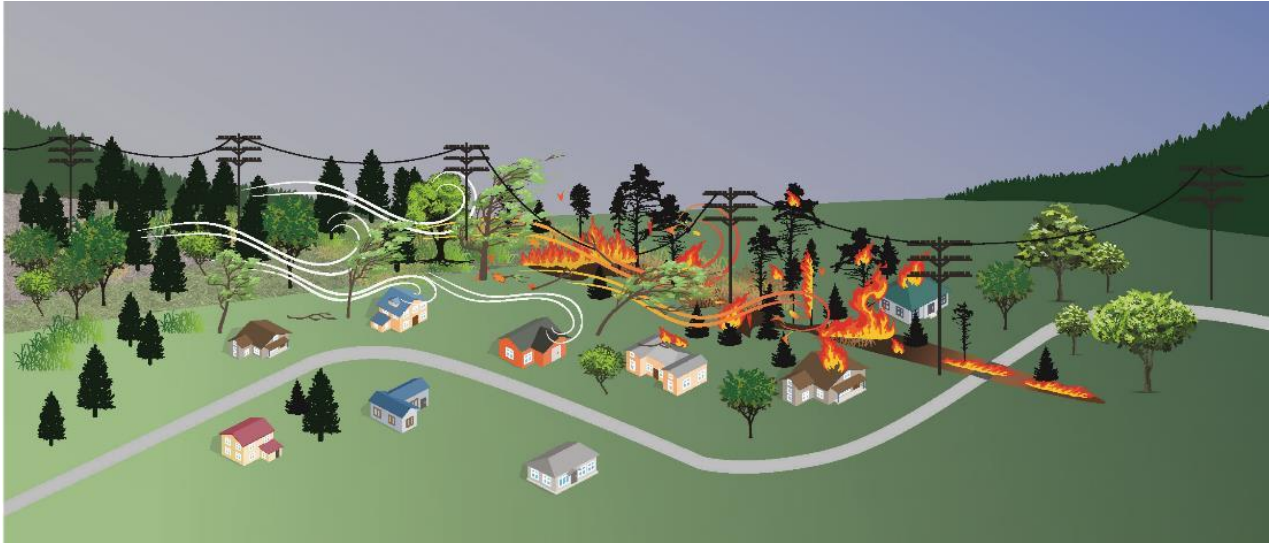
Figure 8. High winds can bring power lines into contact with trees, which can ignite and start a fire. Fire often spreads via wind-driven embers and dry vegetation.
