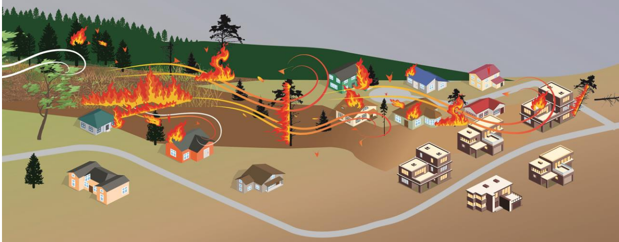
Figure 9. Structure-to-structure ignition occurs when flames, hot gases, embers, or radiant heat from one structure make contact with another structure.
